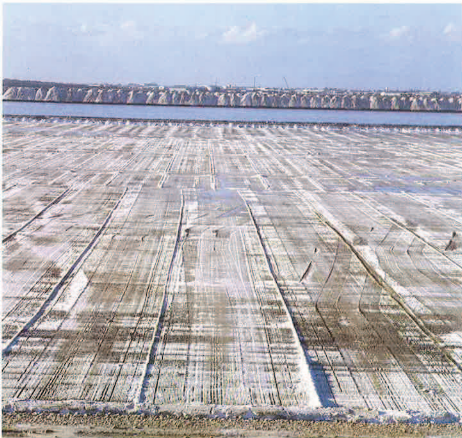
Fig. 5: Crystallising ponds after harvesting. The harvested salt is stored in heaps (see background).
