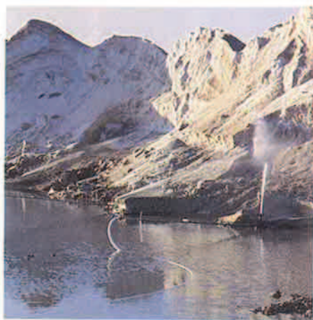
Fig. 1: Water hoses dissolving salt at ICI's Dry Creek field for transport by pipelines to the Osborne Soda Ash works.
