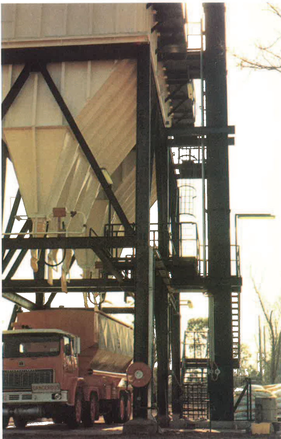
Fig. 1: 2 × 100-tonne capacity bulk ammonium nitrate bins and mobile bulk ANFO unit located at Gregory Mine site, central Queensland.
