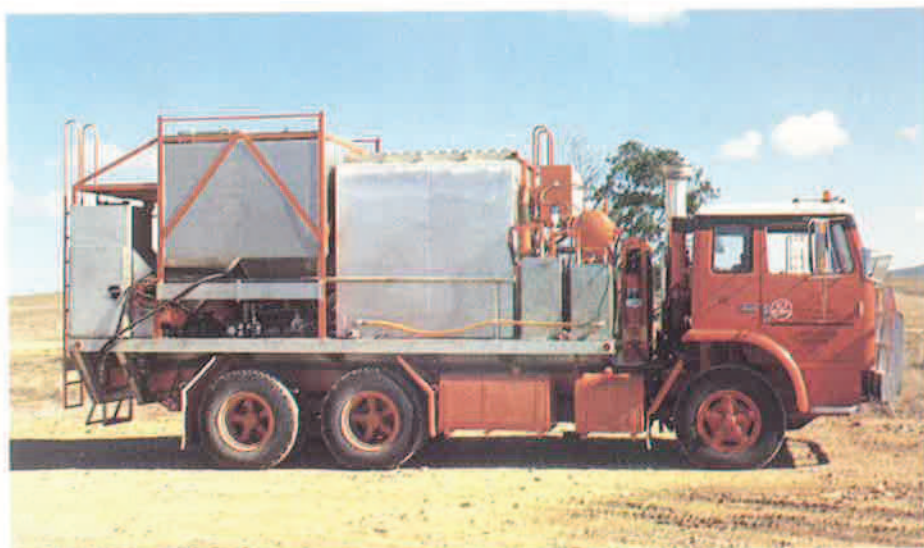
Fig. 2: Mobile bulk Watergel mixing and delivery unit located at Liddell, New South Wales.
