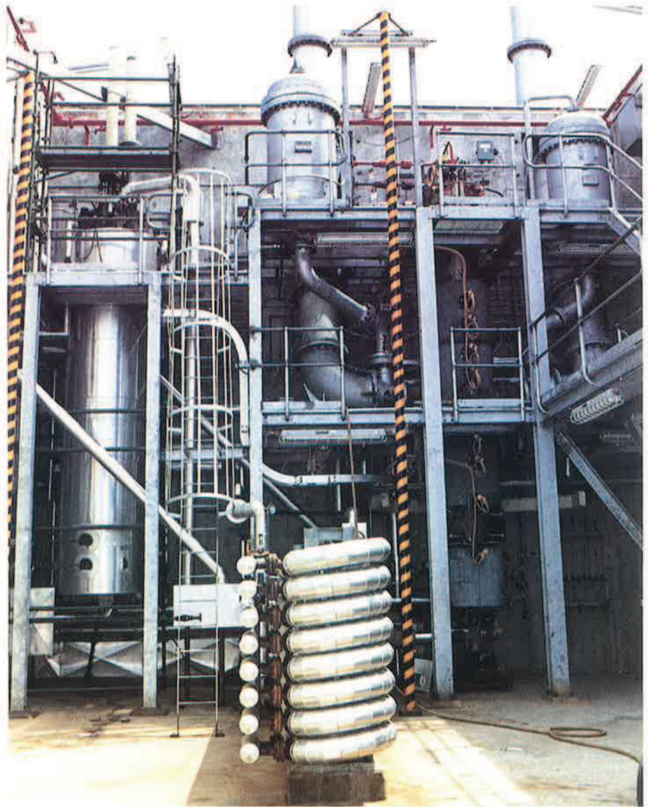
Fig. 2: High pressure reactor bay showing reactor (background right-hand side) and ancillary equipment.
