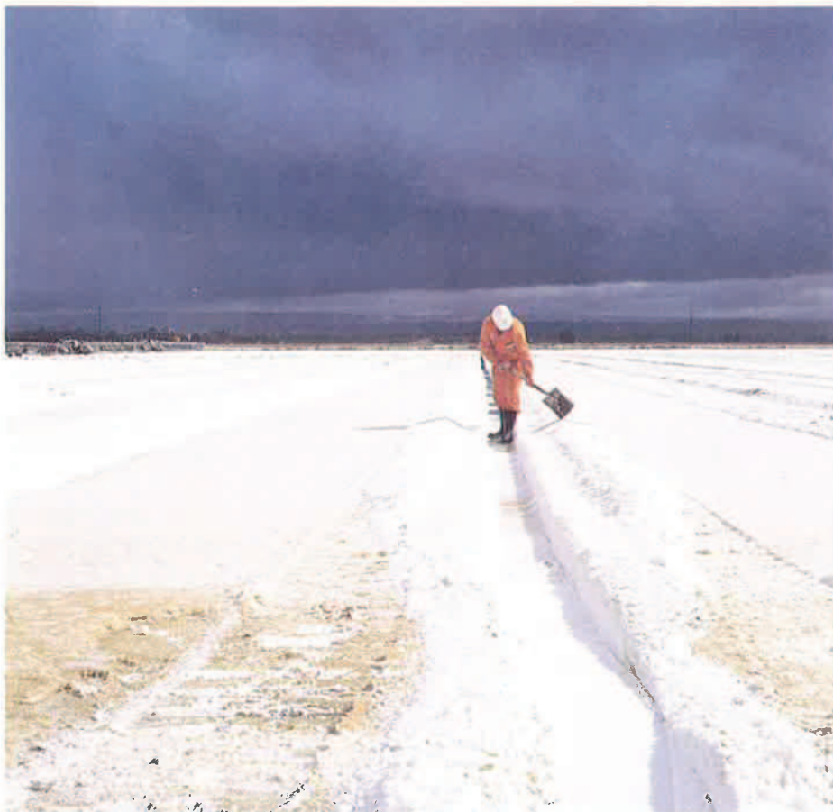
Fig. 4: Clearing drains for removal of unwanted moisture from the salt mass.
