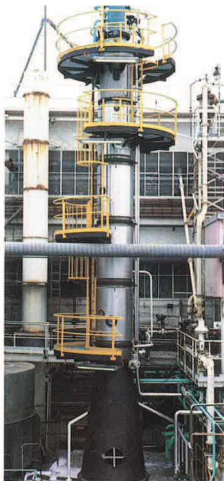
Fig. 2: Continuous PVC Slurry Stripping Column.
